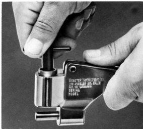
FIG. 4 Adjusting Load on Load Spring
